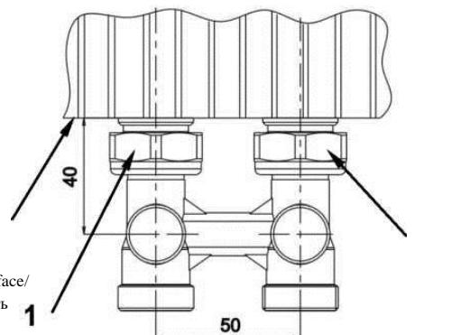
Nuts 1 and 2 must be tightened little by little as pairs and balanced to each other. Avoid to tight with a single turn. In order to achieve perfect leak-tightness, please do not mount the valve stressed and inclined. Tightening moment should not be more than 25 Nm. While assembling angle type H-valve product to the radiator, take care to ensure the distance between radiator bottom surface and control spindle axis is 43 mm.
